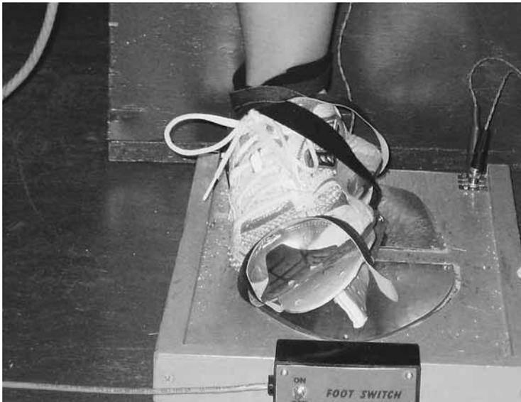
**Figure 4** — Lateral border of the outer sole contacting the landing area, indicating that the participant has completed the 25° of inversion.
